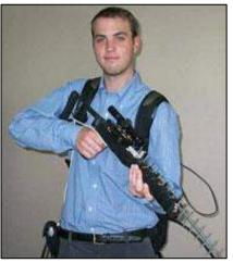
"...BlueSniper rifle, a yagi-antenna and scope affixed to a gun-like stock that this week broke a distance record for BlueSnarfing... by slurping data from a Nokia 6310i from 1.1 away (2 Km) away..."
