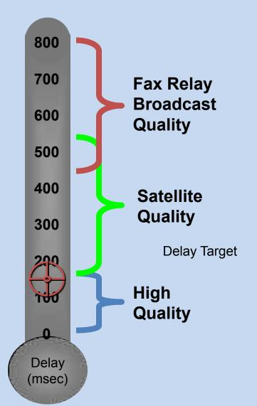
Many factors that contribute to the overall delay are fixed: -Codec delay -Hardware delay -Processing delay -Network physical delay
