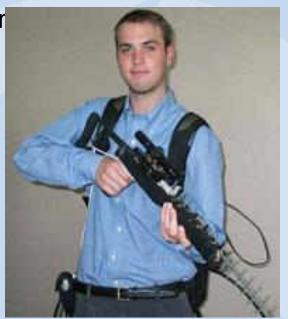
"...BlueSniper rifle, a yagi-antenna and scope affixed to a gun-like stock that this week broke a distance record for BlueSnarfing... by slurping data from a Nokia 6310i from 1.1 away (2 Km) away..." Wired News Aug2004
