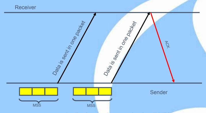
Application data is accumulated until MSS
